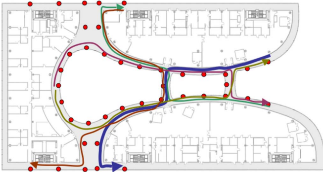
Fig. 9. Forty one stationary sensors (marked with red circle) distributed over 65 \times 100 \text{ m}^2 and moving paths of mobile sinks in the Clark building at Stanford University. Ten different moving paths, including the opposite direction, are explored while a mobile sink carries a sensor device and communicates with the networks.
