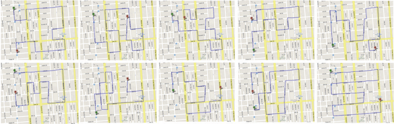
FIGURE 3: Moving paths of mobile vehicles (including the opposite direction as well). A total of 20 vehicles move over the network (as in Figure 2) at a constant speed of 30 km/h with regular time schedules while getting connected to stationary ad hoc nodes.
