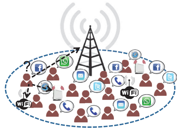
Fig. 1. Dynamic cell selection problem for data offloading in heterogeneous networks of a macrocell, femtocells, and Wi-Fi APs under an overload situation.
