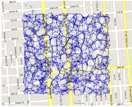
(a) Connectivity graph over 716 sensor nodes where links are shown for PRR > 75%.
